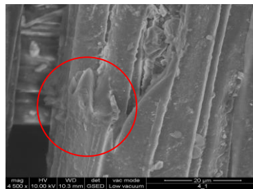
Fig. 2: SEM micrograph of the fibroin microstructure in sample S1, bar: 20 \mu\text{m}
